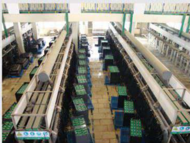
Battery Acid Recirculation Formation System
